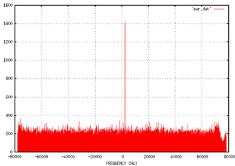
Signal spectrum with 1-sec integration reproduced from data in RDEF format at JAXA
