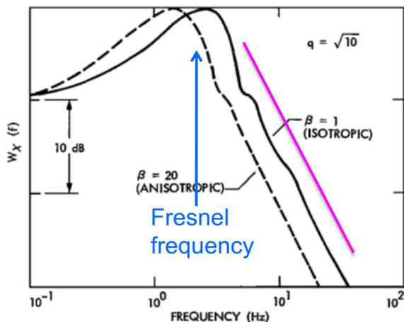
Fig. 1. Model S band log-amplitude power spectra, calculated for the geometry of the 1978 DOY 356 entry occultation. Curves are computed for a 'defocusing attenuation' of 10 dB, Kolmogorov spectrum of refractive index fluctuations, and two values for the irregularity axial ratio  $\beta$ .
